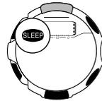
If the **SLEEP** indicator is on the display (either flashing or steady), it means that the display is blank because the watch's Power Saving function has shut it to conserve power. Power Saving automatically turns off the display and puts the watch into a sleep state whenever your watch is left in an area where it is dark for a certain period.
