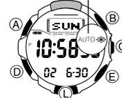
The backlight uses an EL (electro-luminescent) panel that causes the entire display to glow for easy reading in the dark. The watch's auto light switch automatically turns on the backlight when you angle the watch towards your face.
