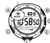
The backlight uses an EL (electro-luminescent) panel that causes the entire display to glow for easy reading in the dark. The watch's auto light switch automatically turns on the backlight when you angle the watch towards your face.
