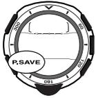
If the **P.SAVE** indicator is on the display (either flashing or steady), it means that the display is blank because the watch's Power Saving function has turned off the display to conserve power. Power Saving automatically turns off the display and enters a sleep state whenever the watch is left for a certain period where it is dark.
