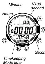
The stopwatch lets you measure elapsed time, split times, and two finishes.
