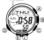
The display of the watch is illuminated using an EL (electro-luminescent) panel for easy reading in the dark. The watch's auto light switch automatically turns on illumination when you angle the watch towards your face.
